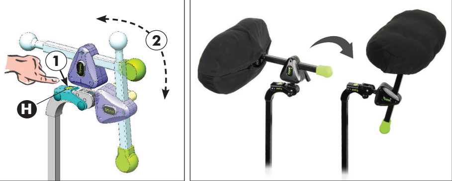
Fig. 6 MATRIX ELAN HEADREST PAD INSTALLATION (SOLD SEPARATELY)
